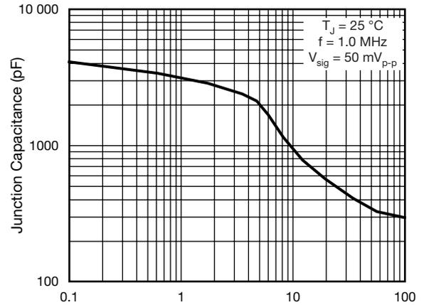
Fig. 5 - Typical Junction Capacitance Per Diode
