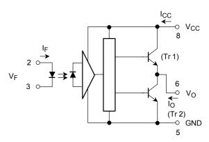
(Note 2 ) A  $0.1\mu F$  bypass capacitor must be connected between pin 8 and 5.
