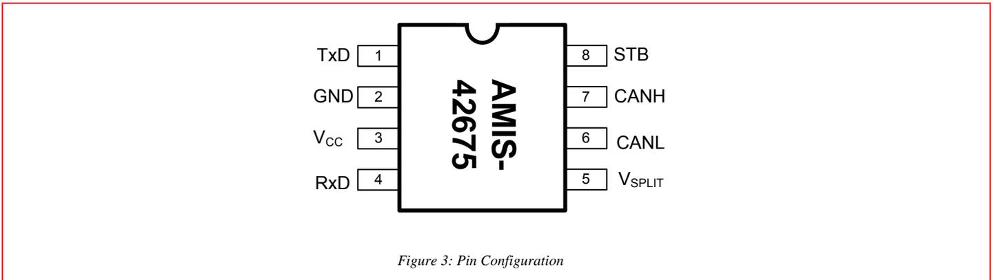
Figure 3: Pin Configuration
