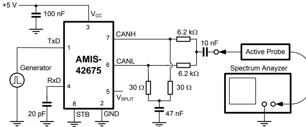
Figure 8: Basic Test Set-up for EME
