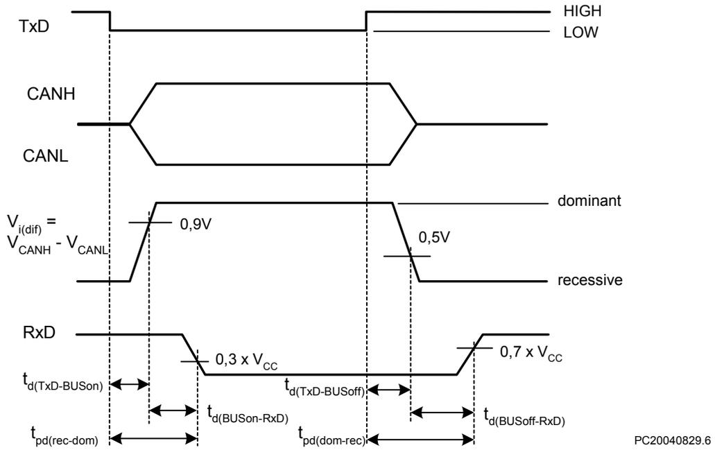
Figure 7: Timing Diagram for AC Characteristics
