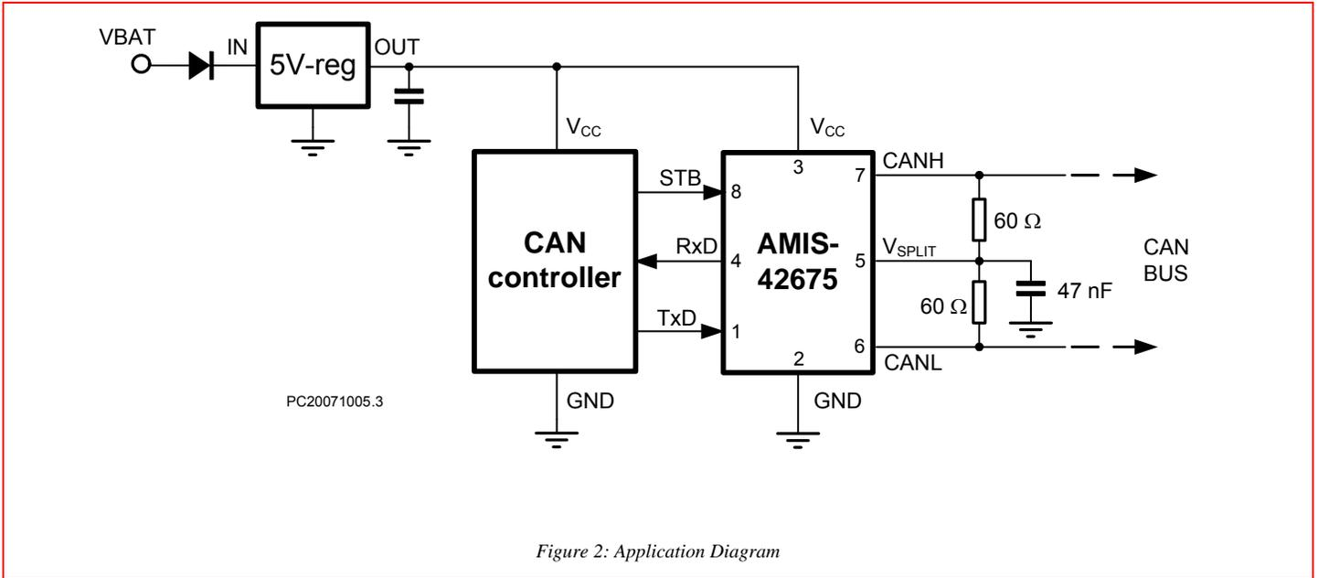
Figure 2: Application Diagram
