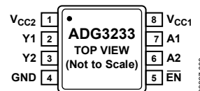
Figure 6. 8-Lead MSOP Package (RM-8)
