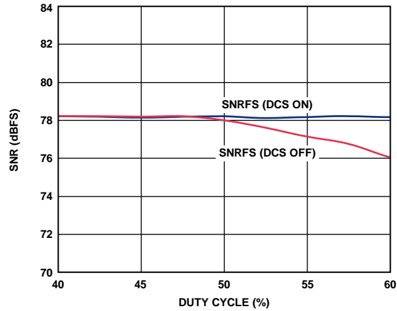
Figure 67. SNR vs. DCS On/Off, V_{REF} = 1.0 V
