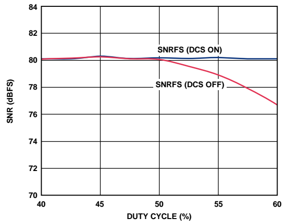
Figure 68. SNR vs. DCS On/Off, V_{REF} = 1.3 V
