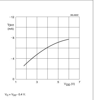
Fig.12 Typical HIGH level push-pull output source current ( $I_{OH1}$ ) as a function of operating supply voltage ( $V_{DD}$ ).
