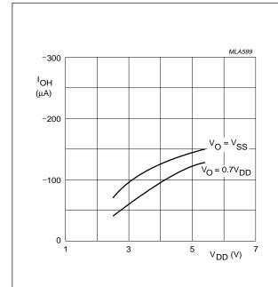
Fig.11 Typical HIGH level pull-up output source current ( $I_{OH}$ ) as a function of operating supply voltage ( $V_{DD}$ ).
