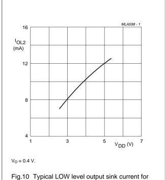
SDA/P2.3 or SCLK ( $I_{OL2}$ ) as a function of operating supply voltage ( $V_{DD}$ ).
