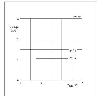
$\label{eq:Fig.8} \begin{array}{ll} \text{Typical supply current in Stop mode} \\ & (I_{DD(stp)}) \text{ as a function of operating supply} \\ & \text{voltage } (V_{DD}). \end{array}$
