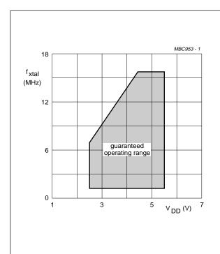
Fig.3 Maximum clock frequency ( $f_{xtal}$ ) as a function of supply voltage ( $V_{DD}$ ).
