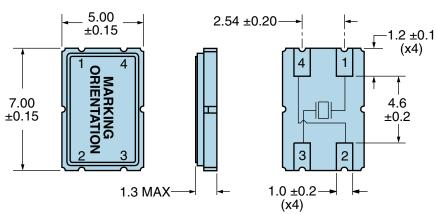
Note: Chamfer and index mark not shown.
