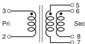
Secondary windings to be connected in parallel on PCB board
