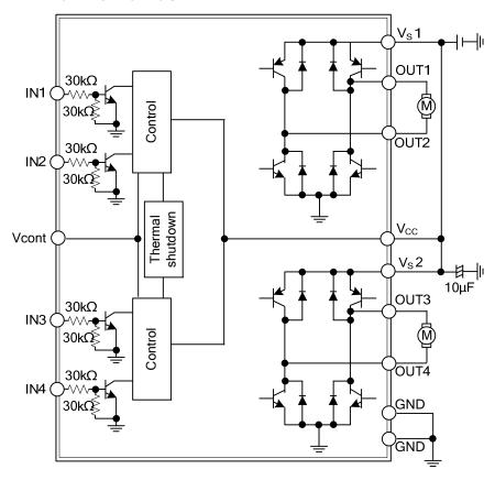
Note: There are no restrictions on the relationship of each voltage level in comparison with the others (regarding which is higher or lower), as long as the voltages applied to  $V_{CC}$ ,  $V_S1$ ,  $V_S2$ , and IN1 through IN4 are within the limits set by the absolute maximum ratings. (Ex:  $V_{CC}=3V$ ,  $V_S1$ , 2=2V, IN1 to IN4=5V)
