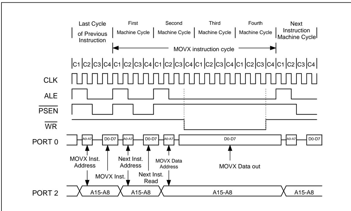
Figure 10. Data Memory Write with Stretch Value = 2
