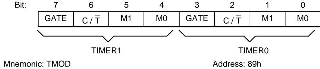
**GATE:** Gating control: When this bit is set, Timer/counter x is enabled only while  $\overline{INTx}$  pin is high and TRx control bit is set. When cleared, Timer x is enabled whenever TRx control bit is set.
