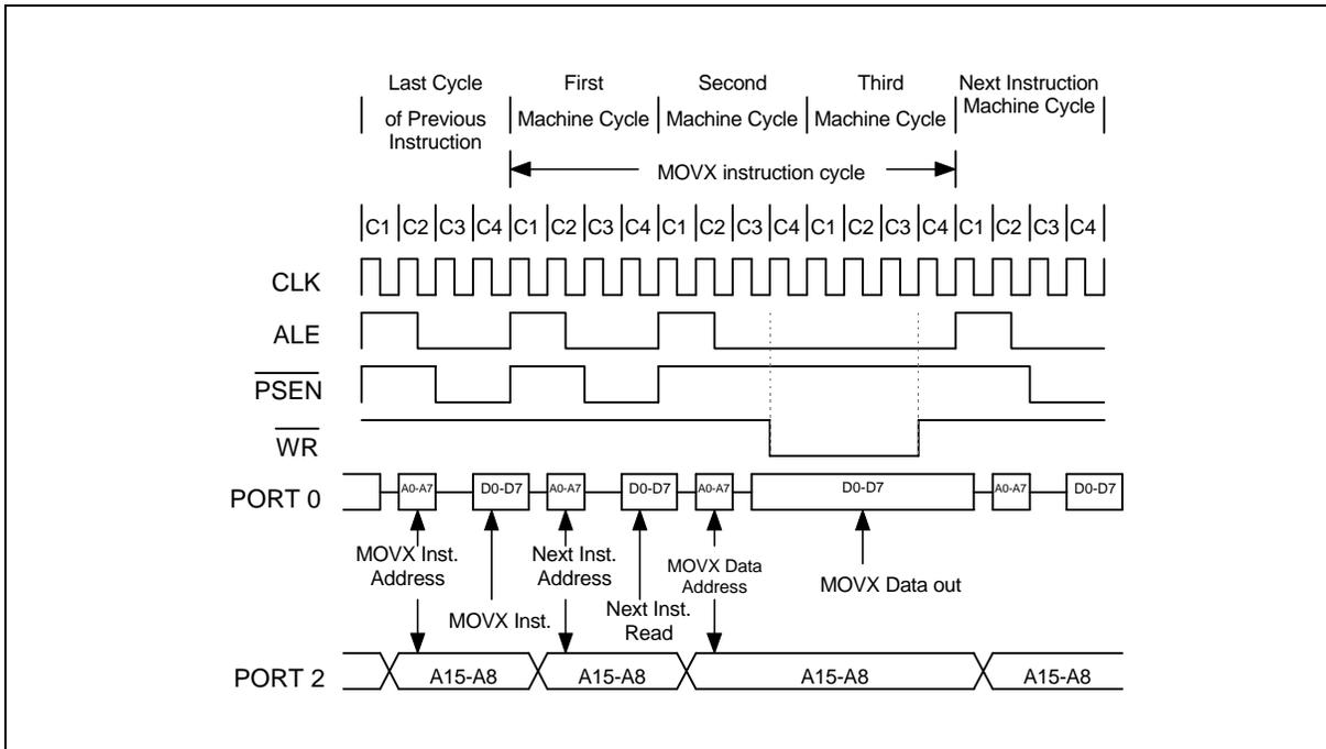
Figure 9. Data Memory Write with Stretch Value = 1
