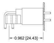
Right Angle Board Mount Female to Straight Board Mount Male (FULLY MATED)
