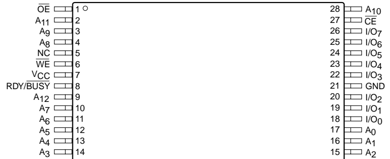
TSOP Package (8mm x 13.4mm) (H13)
