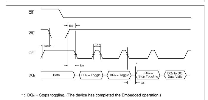
Figure 10 AC Waveforms for Taggle Bit I during Embedded Algorithm Operations
