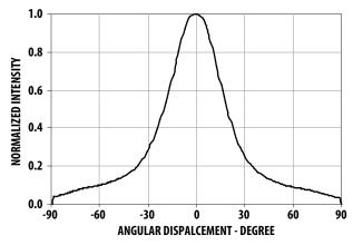
Figure 6. Radiation pattern-Minor Axis
