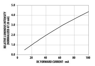
Figure 3. Relative Intensity vs Forward Current
