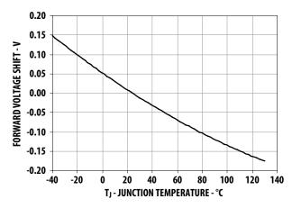
Figure 8. Relative Forward Voltage vs Junction Temperature
