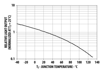
Figure 7. Relative Light Output vs Junction Temperature
