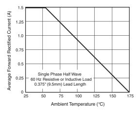
Figure 1. Maximum Forward Current Derating Curve
