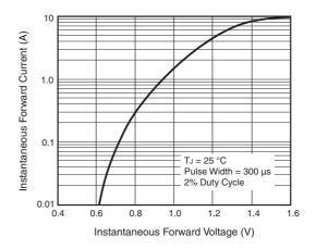
Figure 2. Typical Instantaneous Forward Characteristics
