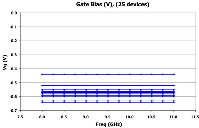
Following test conditions apply for all measured data unless otherwise stated: VD = 8.0V, 4.0A. Pin = +20 dBm, Temp = +25C, Pulsed Duty Cycle = 5%
