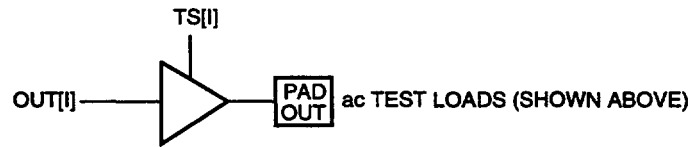
Figure 74. ac Test Loads
