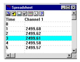
There is one line for each reading. The first two columns show the time and date while the remaining columns show the selected parameters. The scroll bar on the right selects the range of times to display.
