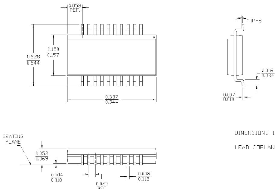
**20-Lead (300-Mil) Molded SOIC S5**
