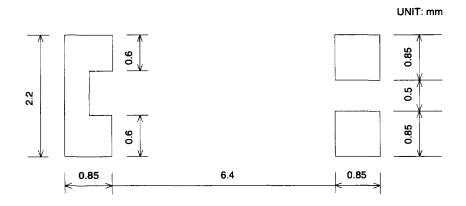
Note: Please make sure that there is no electric wire line under SSP-T6 on the circuit board.
