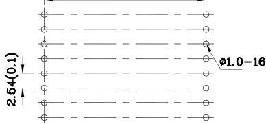
RECOMMENDED PCB LAYOUT 27.94(1.1)
