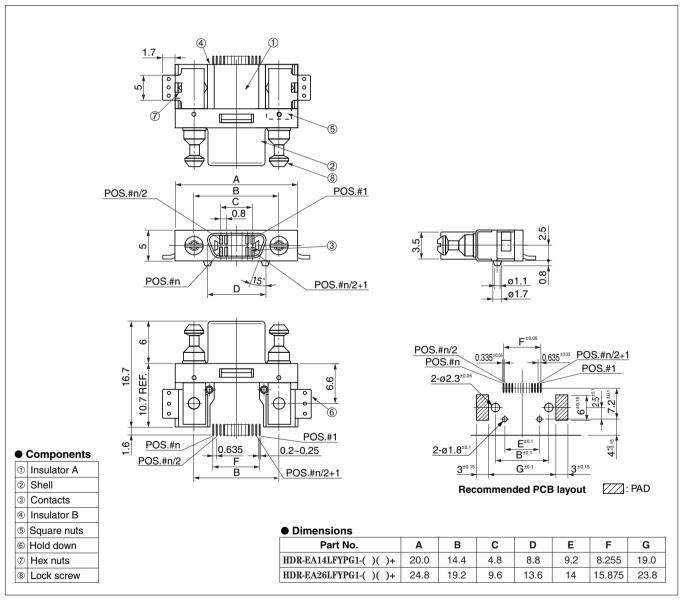
Mating connector: HDR series IDC or solder type male cable connector
