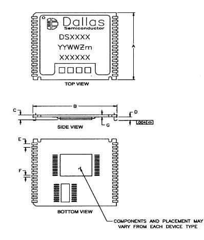
**Note:** Dallas Semiconductor recommends that PowerCap Module bases experience one pass through solder reflow oriented with the label side up ("live-bug").
