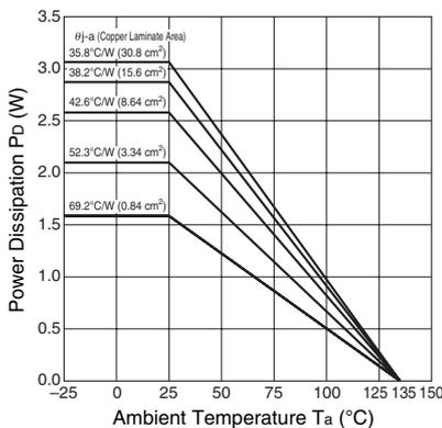
$$P_D = V_O \cdot I_O \left( \frac{100}{\eta\%} - 1 \right) - V_F \cdot I_O \left( 1 - \frac{V_O}{V_{IN}} \right)$$
