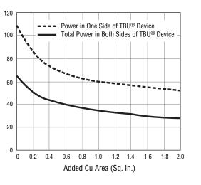
Thermal Resistance vs Additional PCB Cu Area
