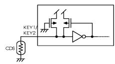
schmitt trigger structure and improves the efficiency of input detection. The pull-high resistor is about 1000K $\Omega$  when the input voltage of KEY1 or KEY2 is lower than  $V_{\rm IL}$ . It turns out to be about 300K $\Omega$  when the input voltage is higher than  $V_{\rm IH}$ .
