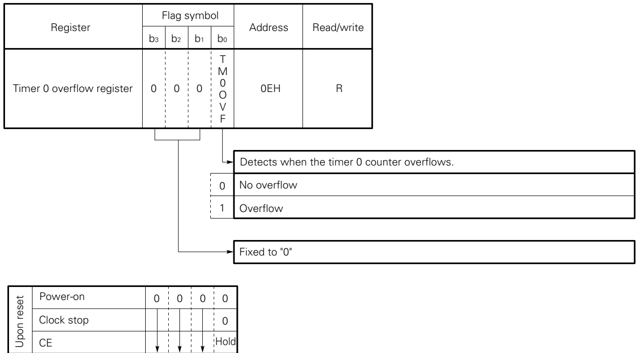
Fig. 12-22 Configuration of the Timer 0 Counter
