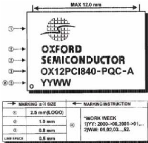
Figure 4: Custom Marking on the 100-pin QFP Package
