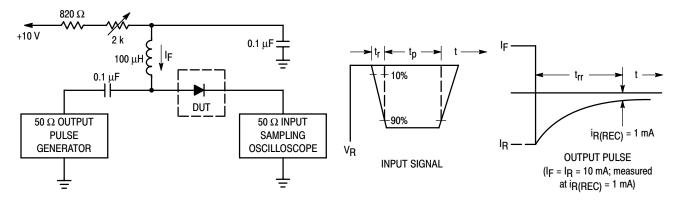
Notes: 1. A 2.0  $k\Omega$  variable resistor adjusted for a Forward Current (IF) of 10 mA.
