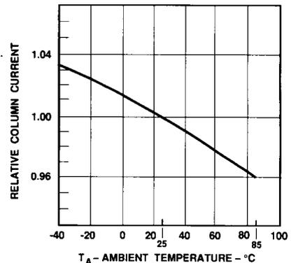
Figure 4. Relative Column Current,  $I_{\text{COL}}$ , vs. Ambient Temperature.
