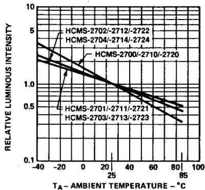
Figure 2. Relative Luminous Intensity vs. Display Pin Temperature.
