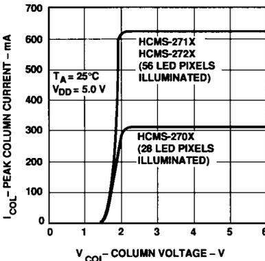
Figure 3. Peak Column Current vs. Column Voltage.
