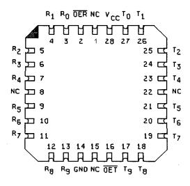
FIGURE 1. <u>Terminal connections</u>.
