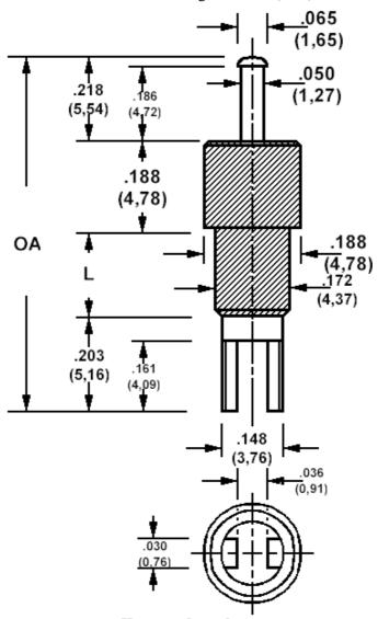
$\frac{571\text{-}4254\text{-}01}{571\text{-}4254\text{-}01} = \frac{571\text{-}4254\text{-}01}{12}$  Basic Part No (XX = panel thickness, YY = plating finish. See tables for options)
