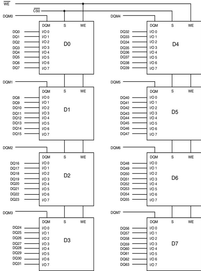
NOTE: DQ wiring may differ than described in this drawing, however DQ/DQMB/CKE/S relationships must be maintained as shown.
