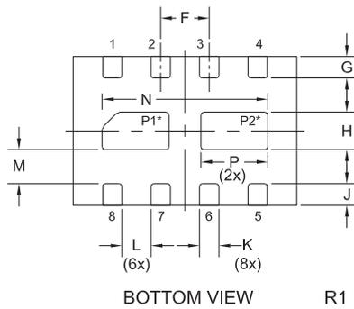
\* Exposed pad P1 common to pins 7 and 8
