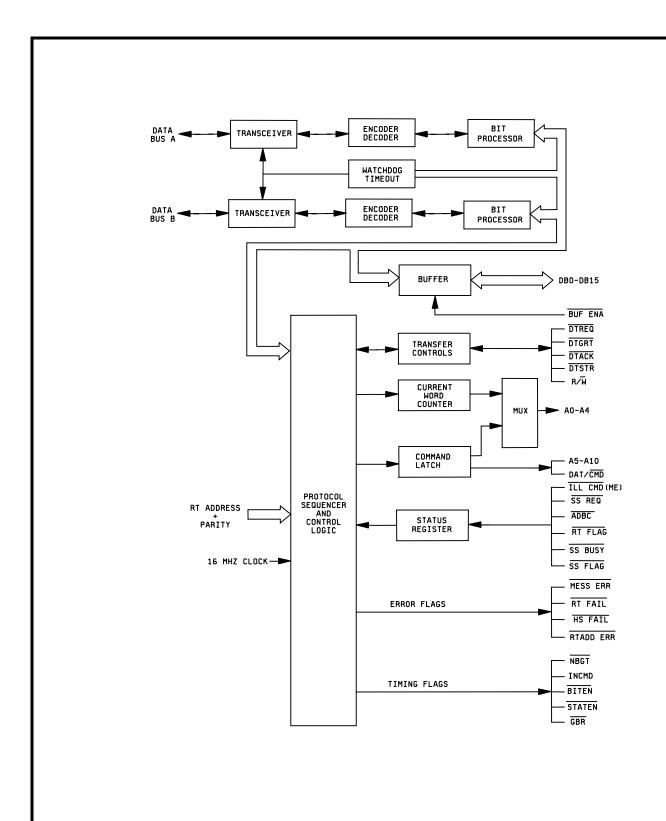
FIGURE 3. Block diagram.
