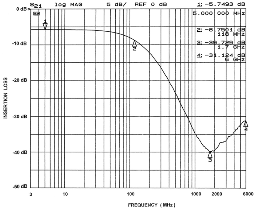
Figure 4. Insertion Loss vs. Frequency (A4-C4 to GND B2)
