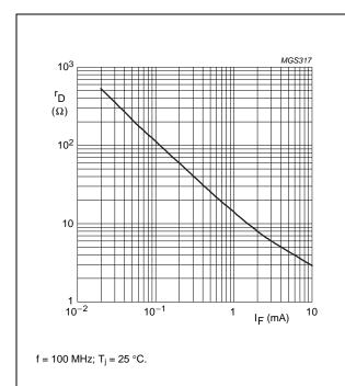
Fig.2 Forward resistance as a function of the forward current; typical values.
