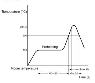
**Note:** The above curve is given on condition that the thickness of the PCB is 1.6 mm.
