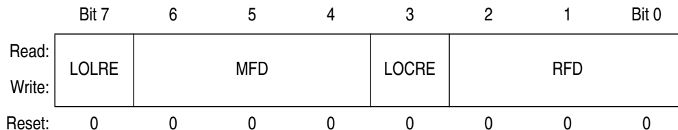
Figure 6-13 ICG Control Register 2 (ICGC2)
