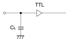
\*1 C<sub>L</sub> includes scope and jig capacitances.
