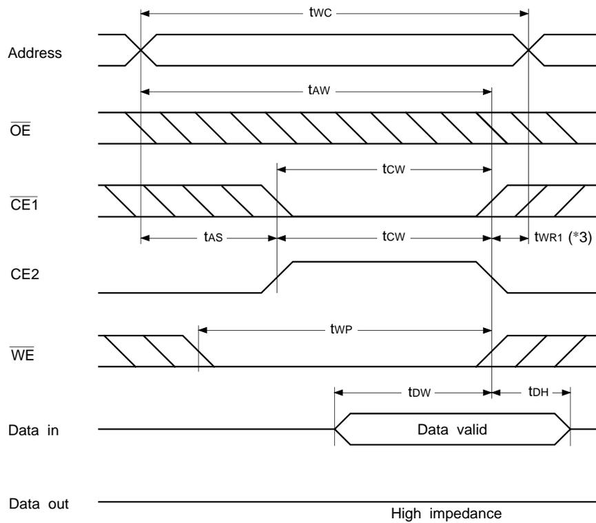
\*1 Write is executed when both  $\overline{CE1}$  and  $\overline{WE}$  are at low and CE2 is at high simultaneously.
