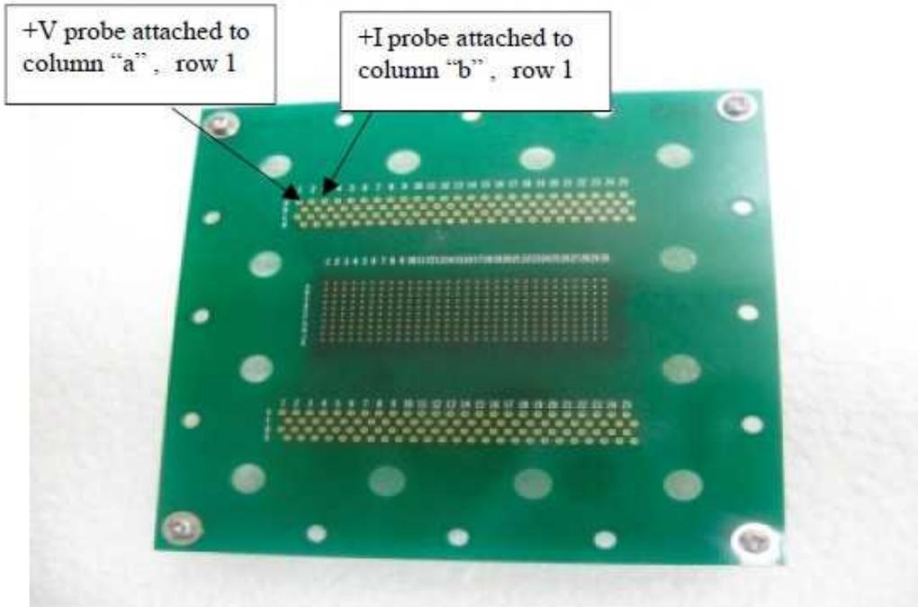
**The -V and -I probes are attached to either side of the common buss.**
