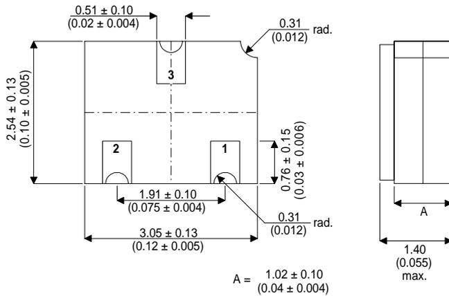
**Bipolar PNP Device in a Hermetically sealed LCC1 Ceramic Surface Mount Package for High Reliability Applications**
