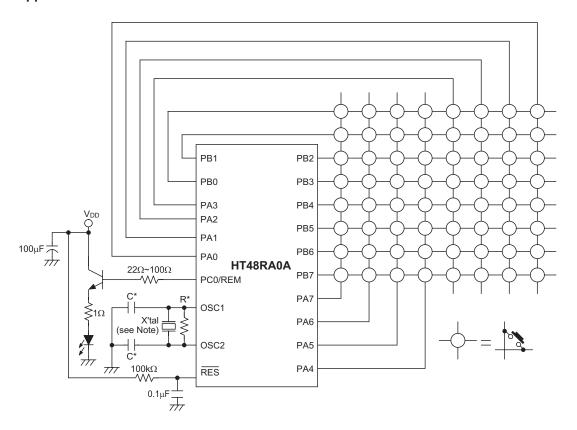
Note: It is recommended that a  $100\mu F$  decoupling capacitor is placed between VSS and VDD.
