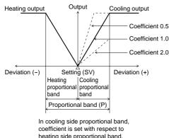
heating side proportional band. (ON/OFF action coefficient 0)
