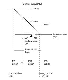
Note : \*ARW: INTEGRAL action is cut when PV is out range of AR value.
