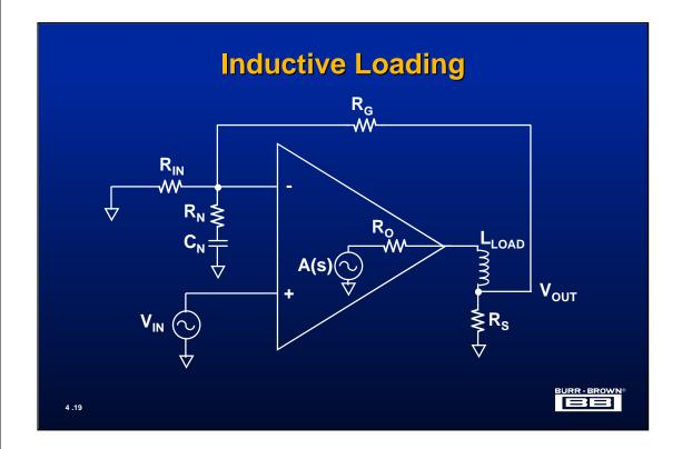
The above schematic shows a typical application for a power op amp when driving an inductive load. Normally the inductor is driven with current as the controlled element. The reason current instead of voltage is controlled is that at DC an inductor is a short circuit and any output voltage would cause the POA to drive a short circuit. Using current control protects both the inductor and the POA from this condition.
