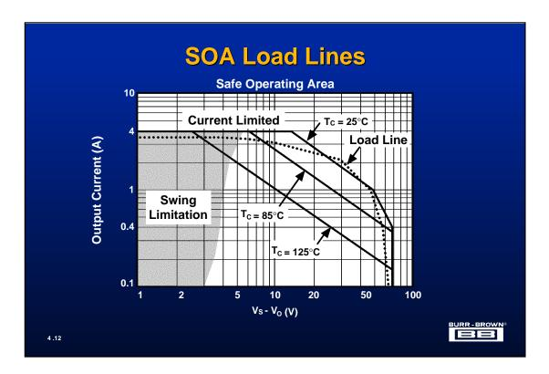
The above graph shows Safe Operating Area or SOA chart for the OPA544. This chart is useful for evaluating the safe electrical and thermal limits of an op amp.
