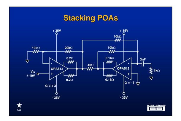
Using a similar master/slave scheme that allows for increasing load current two POAs can be connected as shown above to increase peak-to-peak voltage to a load. The master op amp, on the left, is set for the desired gain and gain polarity while the slave is set for a gain of -1V/V so that its output is the inverse of the master or system gain. This technique not only doubles the available output voltage but also increases the slew rate by a factor of two.
