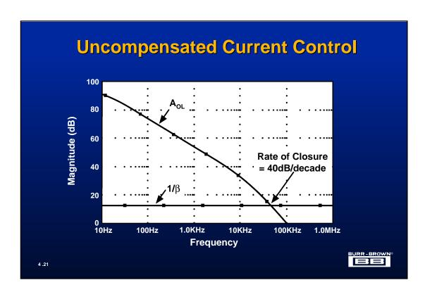
The above plot shows the intersection of the modified open-loop gain characteristic of the current controlled inductor and its  $1/\beta$  plot. As was seen with the uncompensated voltage amplifier, when driving a capacitive load, the rate of closure is 40dB/decade and this circuit is unstable.
