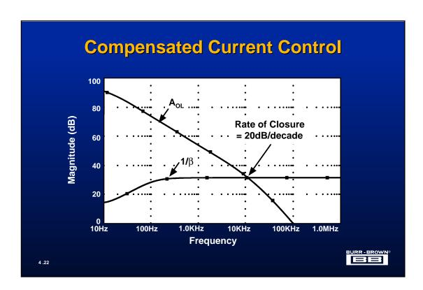
With the addition of the components  $R_N$  and  $C_{N,}$  the 1/ $\!\beta$  plot has been modified to make it rise with frequency before the intersection of the 40dB/decade slope of the open-loop gain of the amplifier. Rate of closure is now 20dB/decade and stability is assured.
