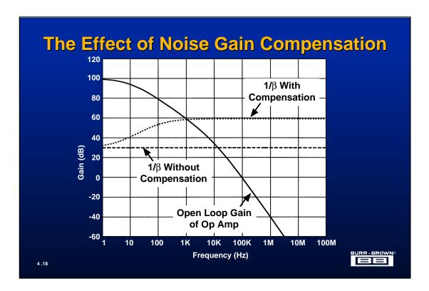
The  $1/\beta$  and open-loop gain characteristics for the capacitive loading application are now shown using the following noise gain components  $R_N = 3.4 k\Omega$  and  $C_N = 0.46 \mu F$ .
