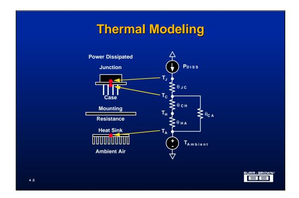
Just because a POA has been selected for an op amp application, that does not ensure it will operate reliably unless a thermal analysis is performed. The data necessary for such an analysis is the thermal resistance of the op amp, the amount of power being dissipated by the amplifier, and the expected maximum ambient temperature.
