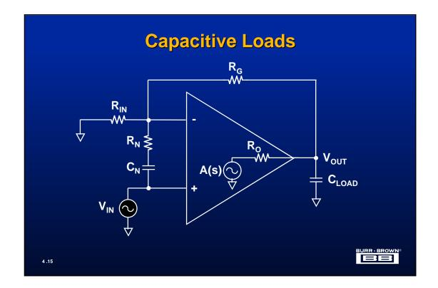
The above diagram shows the pertinent circuit elements used to evaluate the performance of the op amp when presented with a capacitive load. The output impedance has been modeled as simply a resistance of constant value,  $R_{\rm O}$ . While most output impedances also have a reactive element associated with this resistance, it is usually not necessary to include this for a successful stability analysis.
