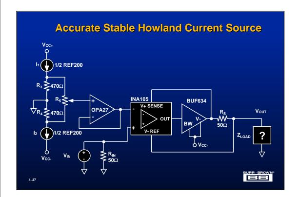
Another application for a POA is the conversion of voltage into an equivalent current. Quite commonly this converted current is used to drive a reactive load. If a POA was used in this configuration with discrete resistors it would be quite common to have stability and accuracy problems. The accuracy problem could be solved with expensive matched resistors. The stability problems could be overcome by noise gain compensation.
