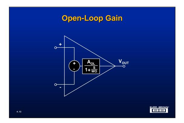
The bode-plot or frequency response of an operational amplifier is almost always shown in a data sheet with either no load or a large resistive load connected to its output. In the typical case, the frequency response is shown to go down 20dB for every decade increase in frequency. This type of response is easily modeled as an amplifier with high DC gain and a single pole filter in series with the amplifier as shown above.
