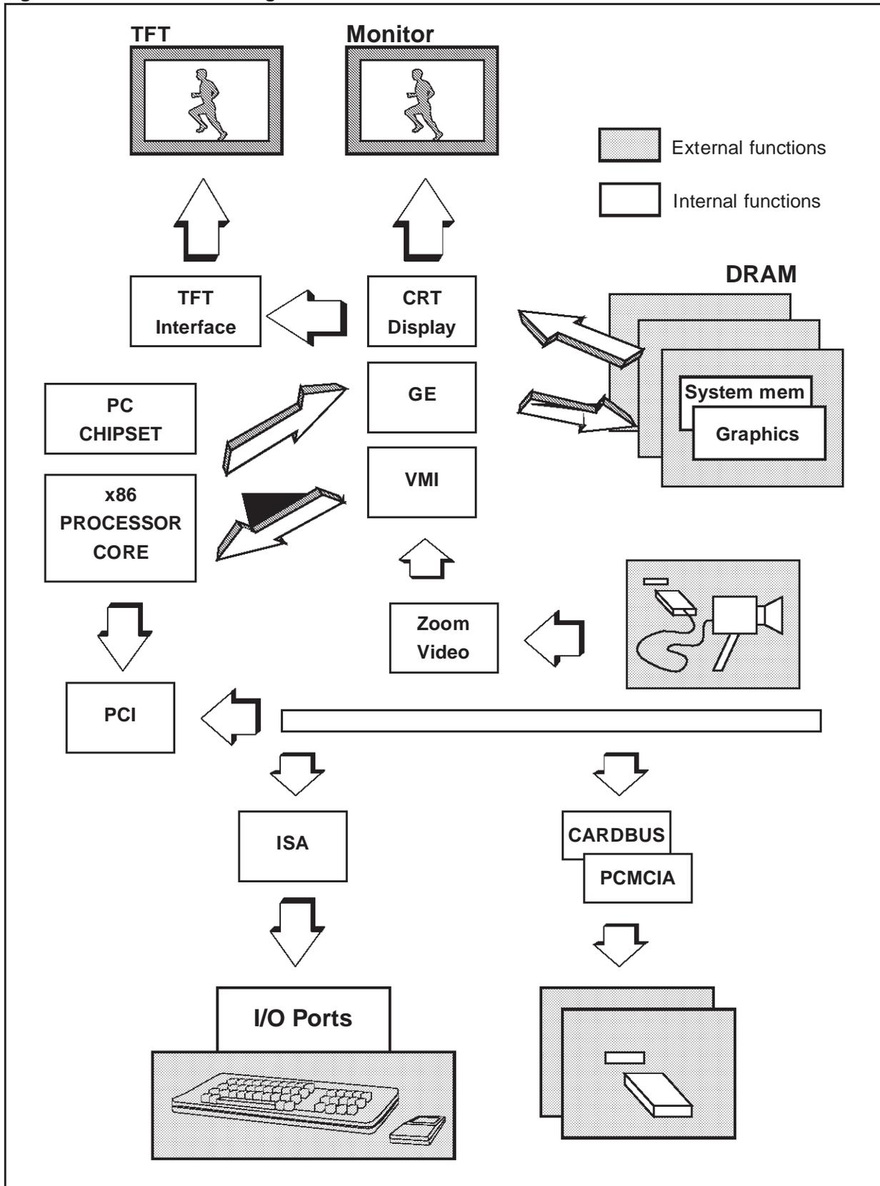
Figure 9. Typical PC oriented Application
