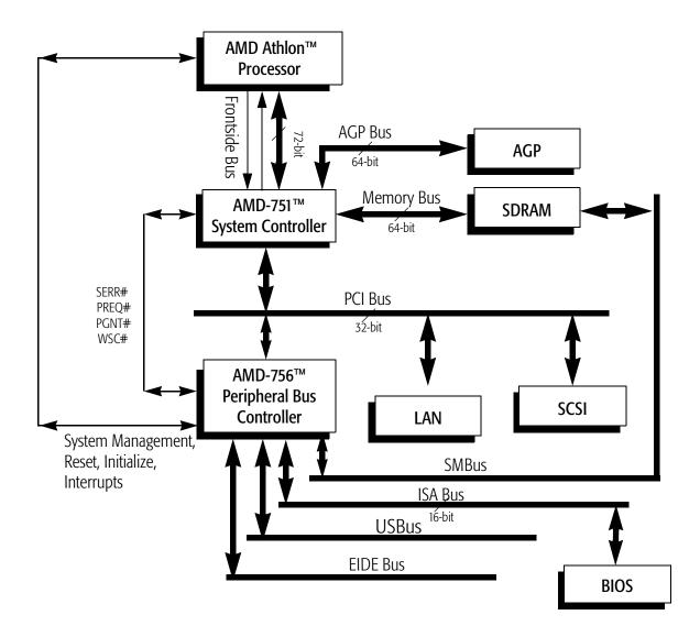
Figure 1. AMD-750<sup>™</sup> Chipset System Block Diagram
