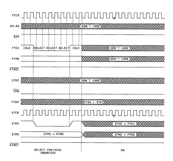
NOTE: The sequence of PTDI bits shown in this figure is only one of many that would produce protocol result soft error.
