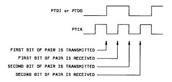
FIGURE 4. Bit-pair timing.
