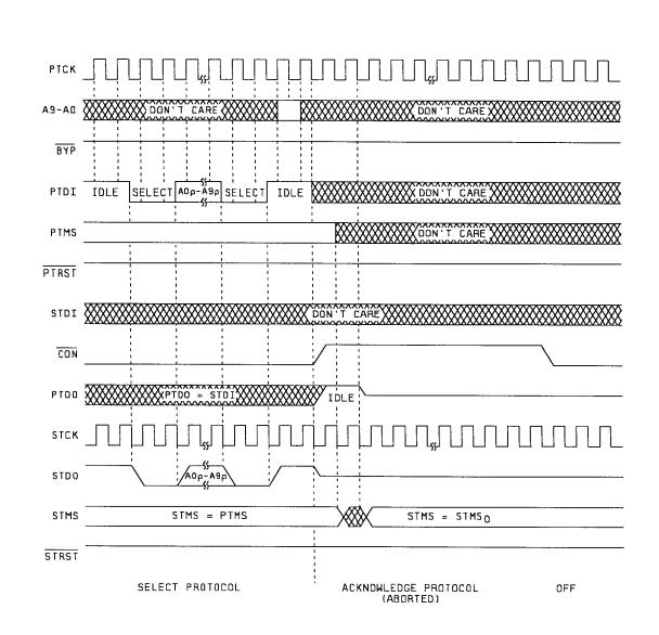
NOTE: The position of PTMS shown in this figure is only one of many that would produce protocol result hard error
