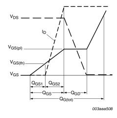
Fig 14. Gate charge waveform definitions
