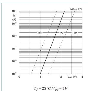
Fig 11. Sub-threshold drain current as a function of
