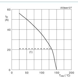
$V_{GS} \geq$  10 V; (1) Capped at 21 A due to wires.
