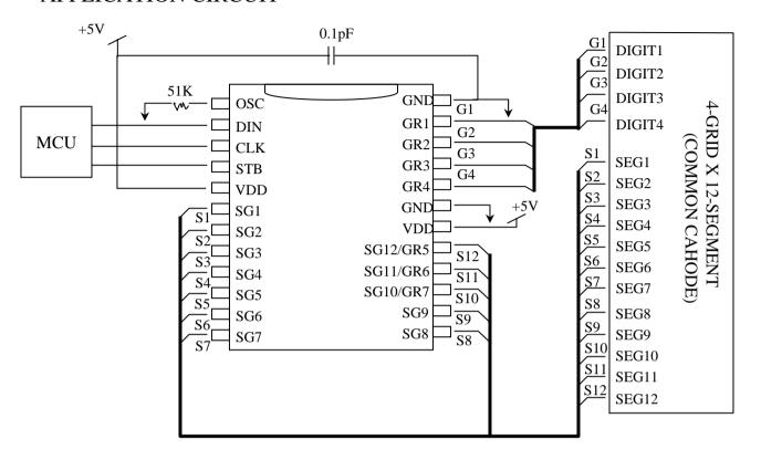
Note: The capacitor (0.1uF) connected between the GND and VDD Pins must be located as near as possible to the LD1207 chip.
